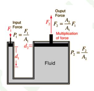
**Hydraulic brakes-** Hydraulic brakes are used in automobiles to stop automobiles. It is work based on Pascal's law.
