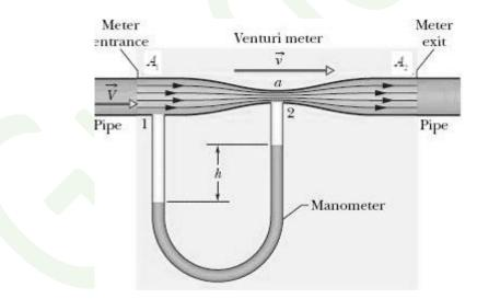
The volume of the liquid flowing per second through the wider tube of area of cross-section A
